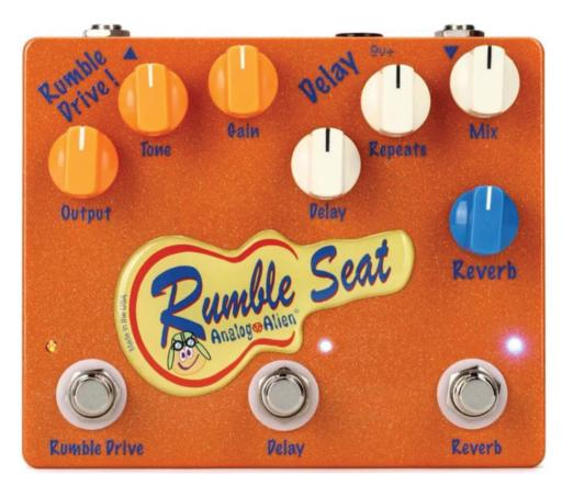
When the Gain control is turned all the way to the left, the Rumble Drive produces very little or no gain at all. At this setting, you can use the Rumble Drive section as a master output and tone control.
